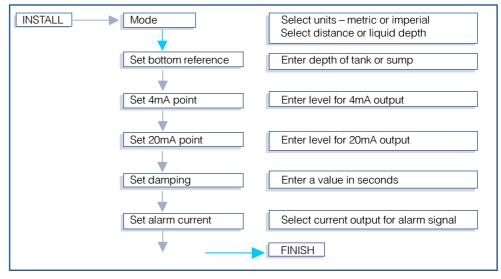
The MSP422 can also be programmed to ignore echoes from false targets, such as ladders or pump tops. If a false target is present, the user can enter the "Lrn" sub-routine of the programme and when the instrument picks-up the false signal, it is told to ignore this from then on.
